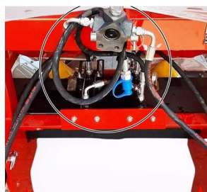
2-Way Automatic Control System
